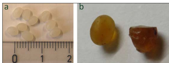
Figure 1: Cellulose beads before (a) and after (b) the functionalization reactions; (b) left: a cut bead prepared for FTIR analysis.
