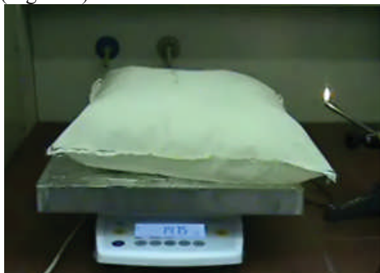
Figure 1. Trial setting according to TB604/1.
