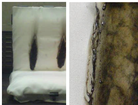
Figure 10. Test sample burned according to BS5852/2.
