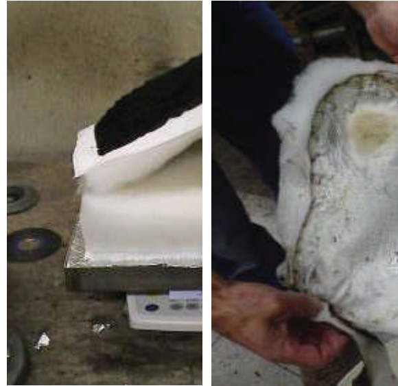
Figure 7. A TENCEL® FILL/polyester fiber blend (left), compared to 100% polyester, burned according to TB604/3.
