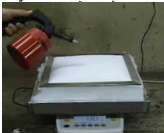
Figure 2. Trial setting according to TB604/3.
