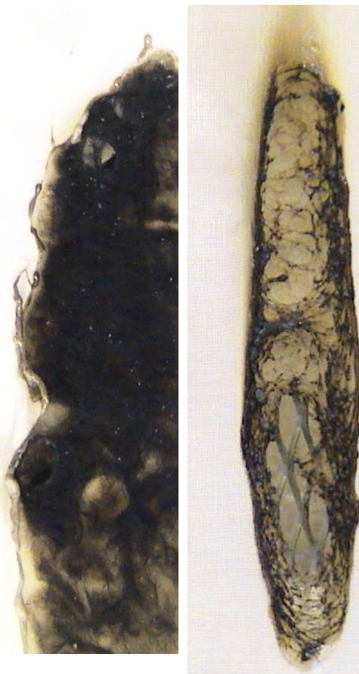
Figure 11. Burning behavior of TENCEL ® FILL/polyester 50:50 blend (left) in comparison to 100% wool (right).
