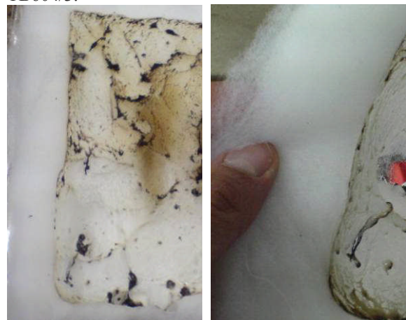
Figure 9. A 100% polyester sample burned according to TB604/3 using a protective barrier fabric.
