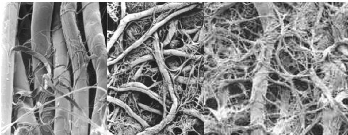
Figure. 6 – Increasing fibrillation of Tencel®
