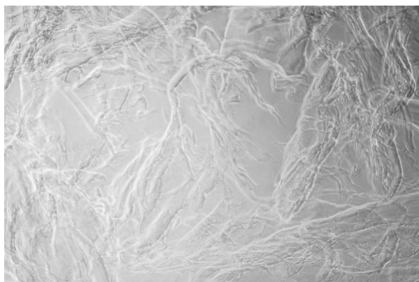
Figure 6. Microscopic picture of the precipitation of a solution of cellulose in BMIMCl in water
