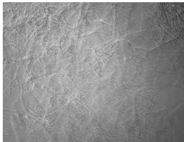
Figure 5. Microscopic picture of the precipitation of a cellulose solution in NMMO hydrate in water
