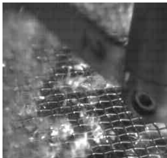
Figure. 4 - Tencel® Fibres in an Airlay Chamber
