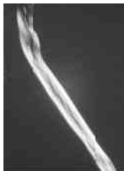
Figure 11. Lyocell fiber treated with the mixture of 0.26 M DMDHEU and 0.19 M MgCl_2 at room temperature and then splitted by shear method (split number is 2)
