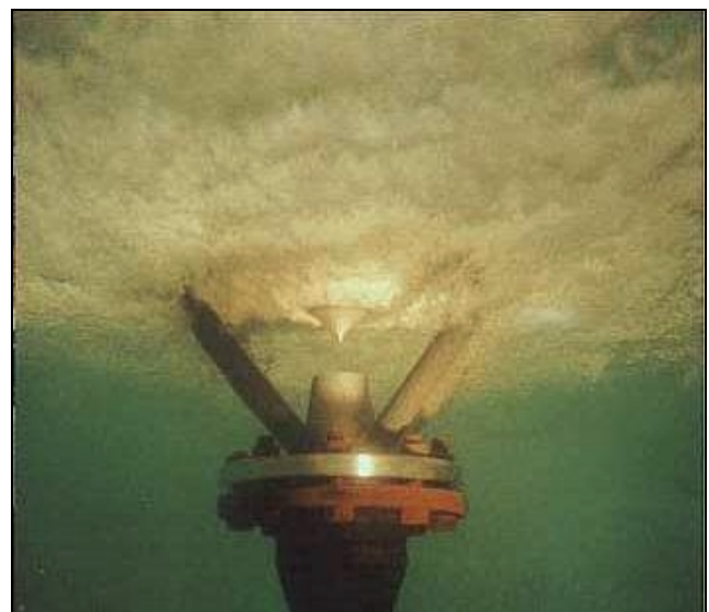
Figure 5. Aeration system: radial flow.
