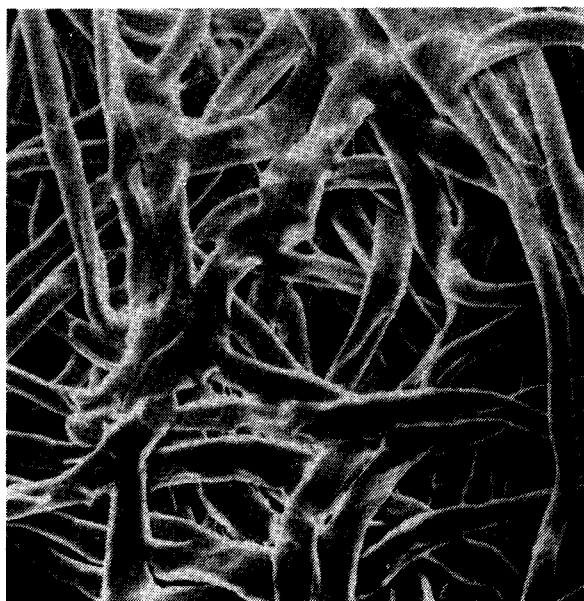
Fig. 9: Bonded spot of a coverstock from a PP fibre not suitable for thermal bonding (220 x)
