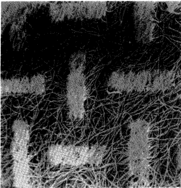
Fig. 3: General view of a bonded coverstock produced from a PP fibre specially designed for thermal bonding (25 x)
